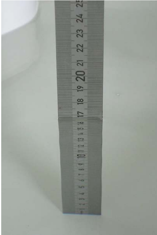
Fig. 11: Liquid depth for 2.4 GHz WLAN.
