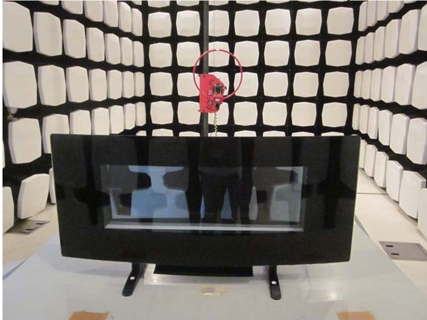
Measurement of Radiated Emission Test Set Up
