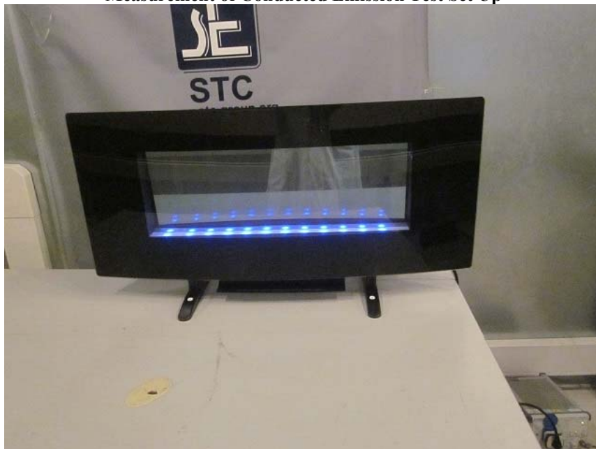
Measurement of Conducted Emission Test Set Up
