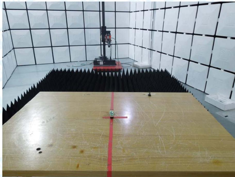
**Photo of Setup for Radiated Emission (Below 1 GHz)**
