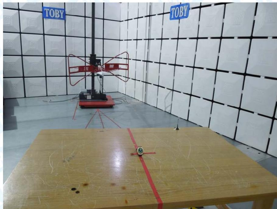
**Photo of Setup for Conducted Emission**
