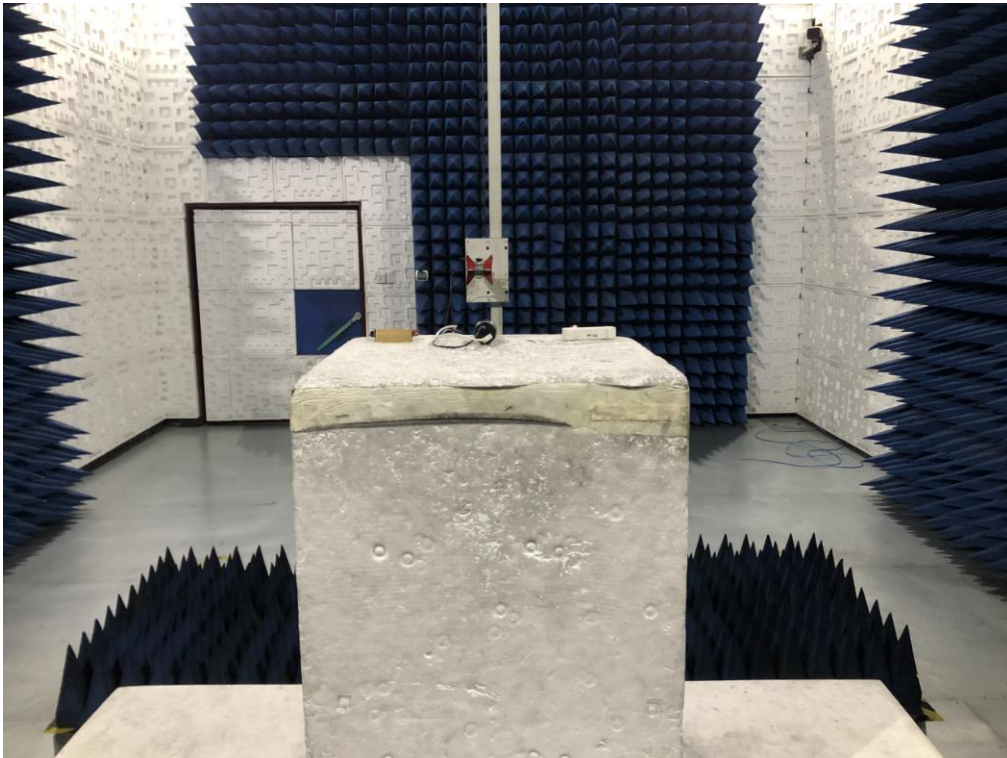
RADIATED EMISSION TEST SETUP ABOVE 1G
