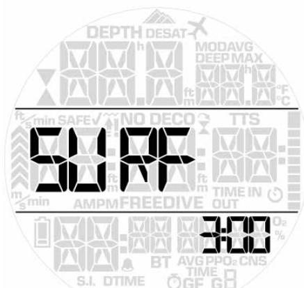
In this menu you can set the duration of the interval from the moment you reach the surface to when the dive computer closes the dive. During this interval you can submerge again and resume the dive. This menu allows you to change the default 3-minute interval to any value between 1 minute and 45 minutes.
