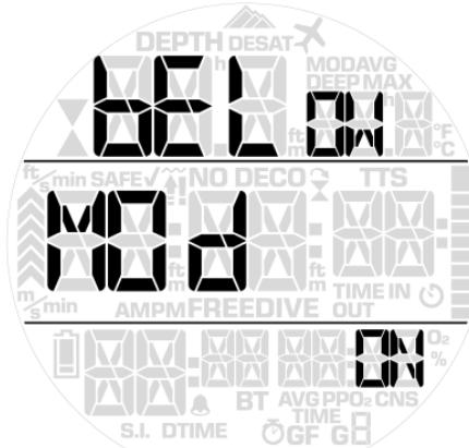
When set to **ON**, Sirius L will allow a switch to a gas at a depth deeper than the MOD of the gas (resulting in an immediate MOD alarm).
