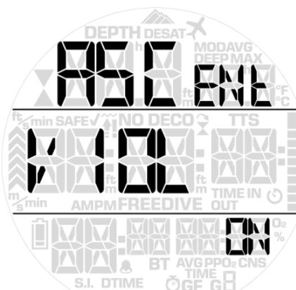
If the ascent rate exceeds 120% of the allowed value over a depth change of more than 20m/66ft, due to the potential of harmful bubble formation, Sirius L locks the computer for 48 hours in order to prevent you from diving again. In this menu, you have the option to disable the locking up of the computer in the event of an uncontrolled ascent.
