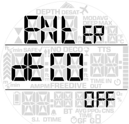
When this is set to **ON**, a warning will alert you when a mandatory decompression stop has been calculated by Sirius L.
