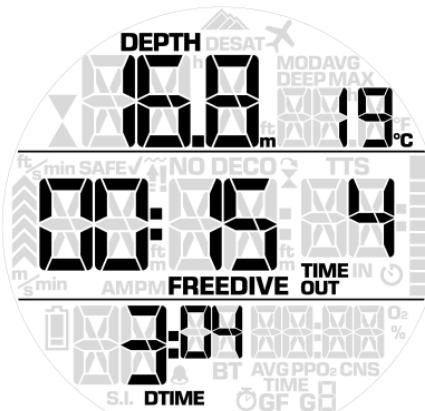
With **TR-SP** the display switches to time of day and current temperature. With **TR-SP** you return to the previous display.
