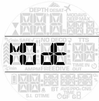
In this menu you define the type of gas you will be breathing during the dive (**AIR** as **SINGLE GAS, NITROX** as **SINGLE GAS, NITROX** as **MULTIGAS**). You can also set Sirius L to **BOTTOM TIMER** or **FREEDIVE**, in which case Sirius L will show only time, depth and temperature: it will not carry out any decompression calculation and it will not show any warnings and alarms.
