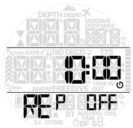
The countdown timer can be set to repeat automatically until it is stopped. With **TR-LP** you start the process of setting the timer. At first the minutes of the time will blink: modify with **TR-SP** or **BR-SP** (up to 60 minutes maximum) and confirm with **TR-LP**.
