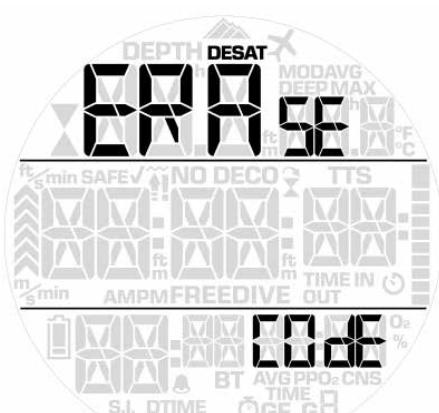
Sirius L allows you to reset the desaturation in the computer. Any tissue saturation information from a recent dive will be reset to zero and the computer treats the next dive as a non-repetitive dive. This is useful when the computer is loaned to another diver who has not dived in the last 24 hours.
