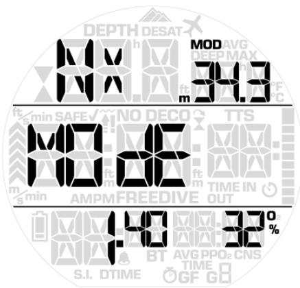
Once inside this menu, use **TR-SP** or **BR-SP** to change the  $O_2\%$ , and watch how this affects the maximum operating depth (MOD). Then with **TR-LP** move on to the  $ppO_2\text{max}$  and use **TR-SP** or **BR-SP** to change the value, again noticing how this affects the MOD. **TR-LP** saves the set values and returns to **PRE-DIVE**. Note that if you press **BR-LP** after setting the  $O_2\%$  value, you skip the  $ppO_2\text{max}$  setting and return directly to **PRE-DIVE**.
