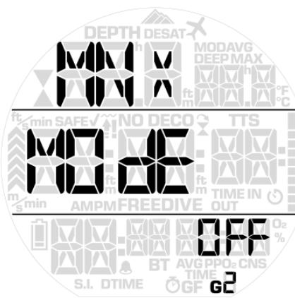
and in the top right corner the MOD of G2 is displayed, also blinking.
