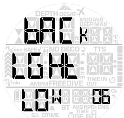
This menu allows you to set the duration of the backlight between 2 and 12 seconds. Default setting is 6 seconds.
