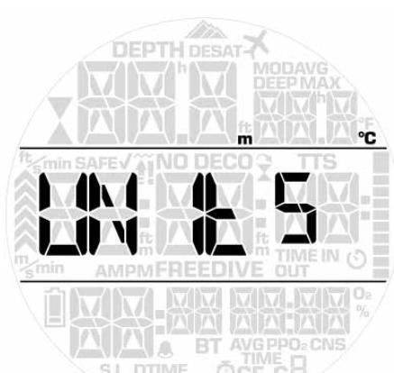
You can choose between metric (depth in meters, temperature in °C), and imperial (depth in feet, temperature in °F).
