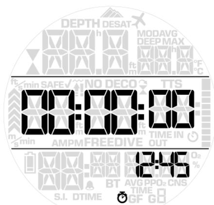
**TR-SP** starts and stops the stopwatch, **BR-SP** resets it, **BR-LP** exits the stopwatch.
