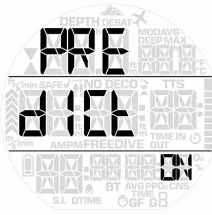
When set to **ON**, Sirius L will consider all gases in the decompression calculation, with switches carried out at the MOD of each gas. When set to **OFF**, the decompression calculation will consider the currently breathed gas only. See Section 11 for more information about the **PREDICTIVE** feature.
