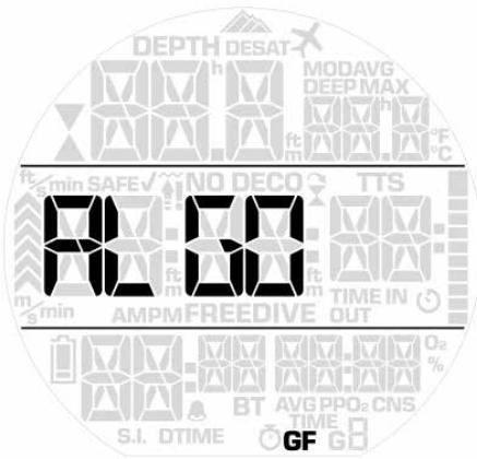
Sirius L employs the unmodified Bühlmann ZH-L16C algorithm with gradient factors. Gradient factors are used to lower the maximum tolerated inert gas pressure in the tissues with respect to Bühlmann's original values. This results in less nitrogen in the body at the end of the dive, which under normal
