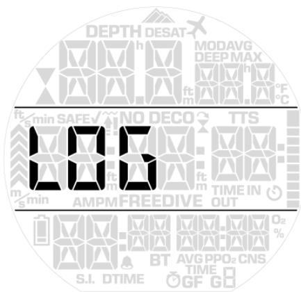
Sirius L can record the profiles of over 100 hours of diving, at a sampling rate of 5 seconds. The information can be transferred to a Smartphone (Mares or MySSI app, via bluetooth). In addition, Sirius L can show most of the information directly on the display. Upon entering the logbook you will see **StAt**. Entering this menu will show the deepest depth, longest dive time and lowest temperature recorded, in addition to the total number of dives and total number of dive hours.
