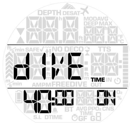
Sirius L allows you to set a time alarm, triggering also a warning at half of the set time limit. The default value is **OFF**. Using the button, you can set the value between 20 and 90 minutes in 2-minute increments. Upon reaching half of the set limit, the dive time will blink until you hit any button to acknowledge it. Upon reaching the set time limit, the dive time again blinks until you hit any button to acknowledge it.
