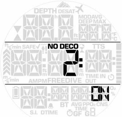
When this is set to **ON**, a warning will alert you when the NO STOP time reaches 2 minutes.
