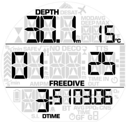
With **TR-LP** you enter the session and see max depth and sequential counter of the immersion, dive time, surface interval prior to immersion and minimum temperature of the immersion. With **TR-SP** you advance to the next immersion in the session. With **BR-LP** you return to the list of dive logs.
