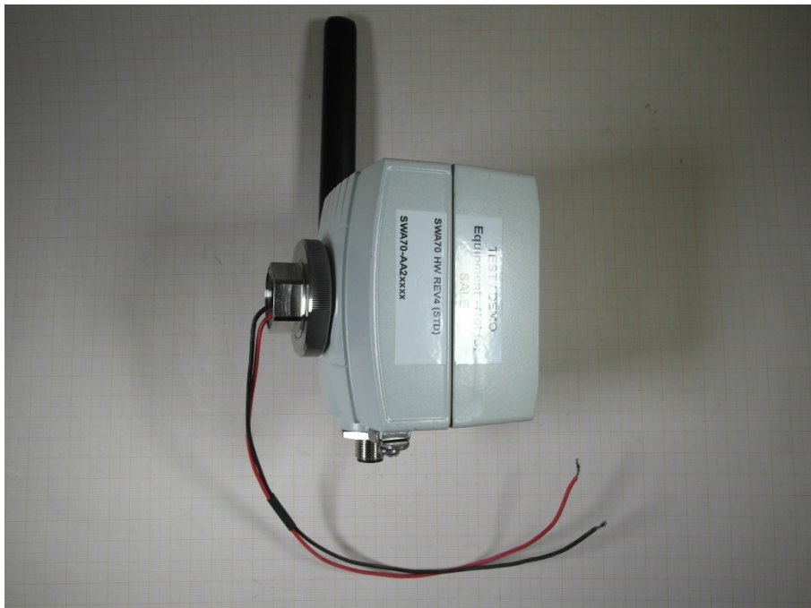
Photo 16: metal housing (non-ex version)
