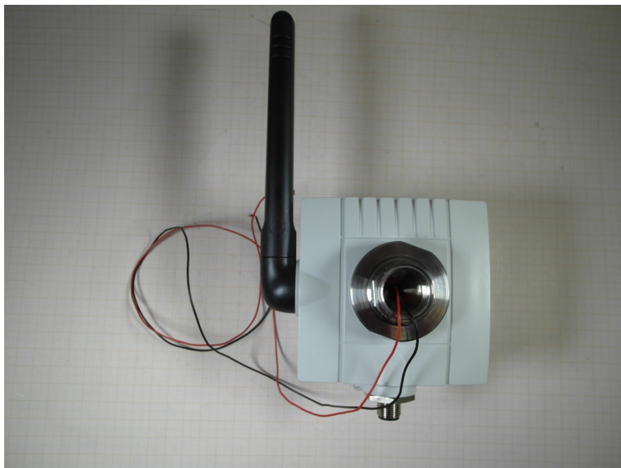
Photo 20: plastic housing (non-ex version)
