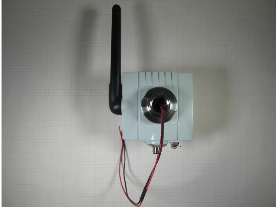
Photo 15: metal housing (non-ex version)
