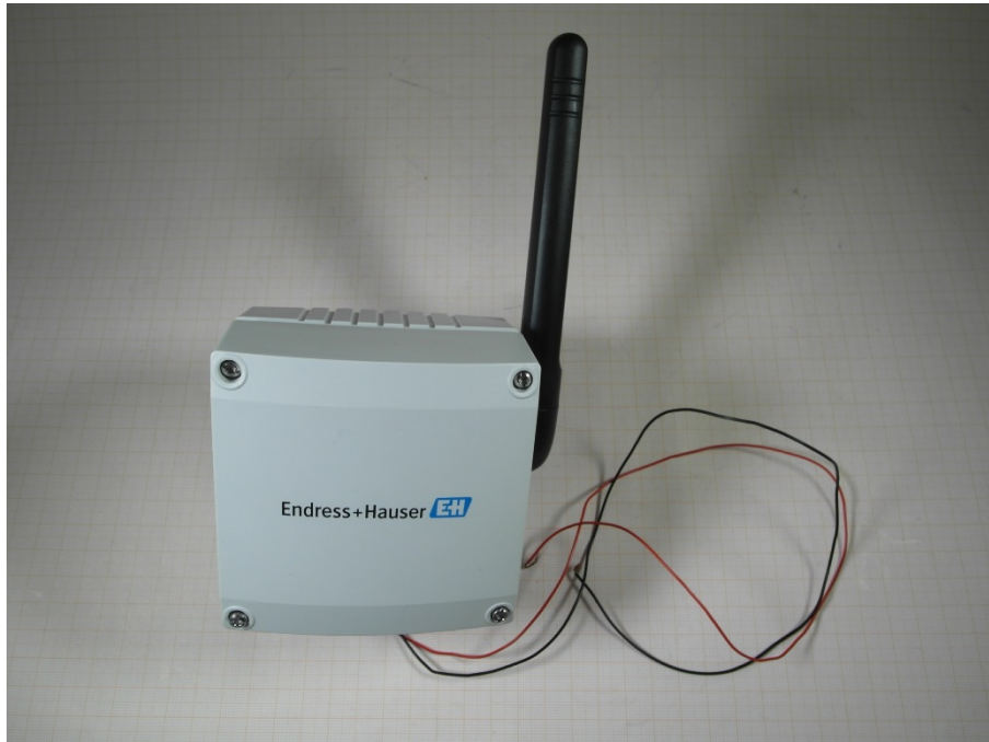
Photo 19: plastic housing (non-ex version)
