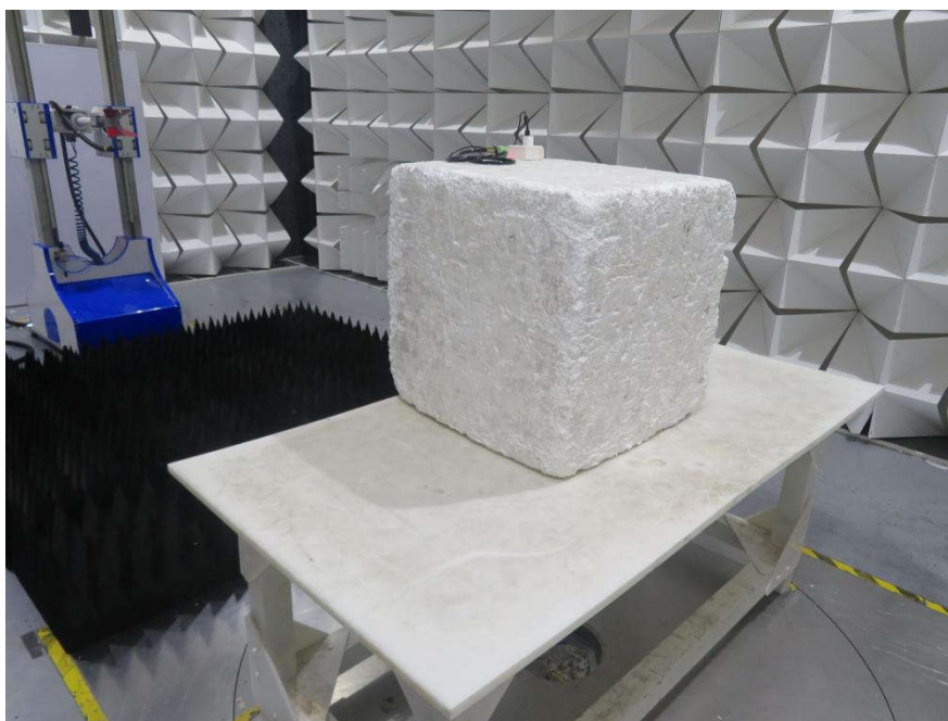
Radiated spurious emission Test Setup-3(Above 1GHz)
