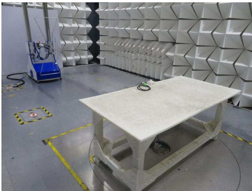
Radiated spurious emission Test Setup-2 (30MHz~1GHz)
