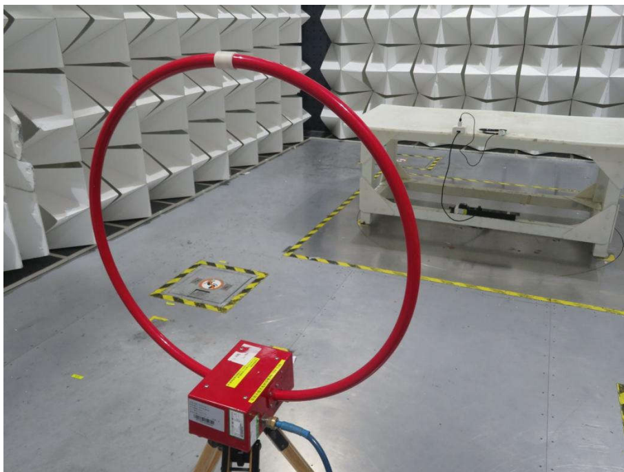
Radiated emission Test Setup-1(9kHz~30MHz)
