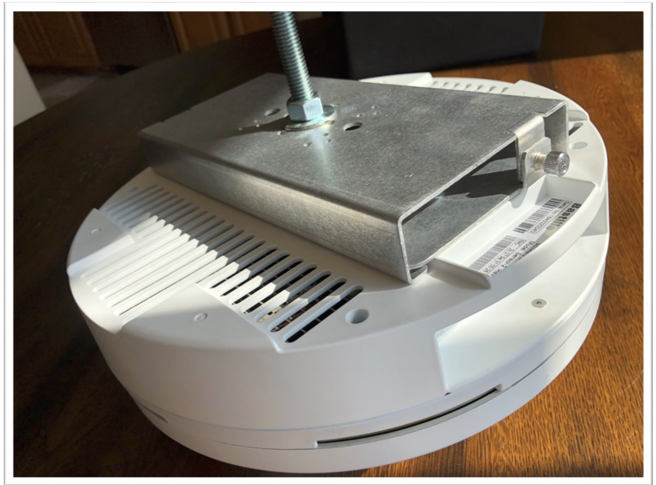
Figure 10. Mounting Plate Fully Inserted to Adapter Plate.
