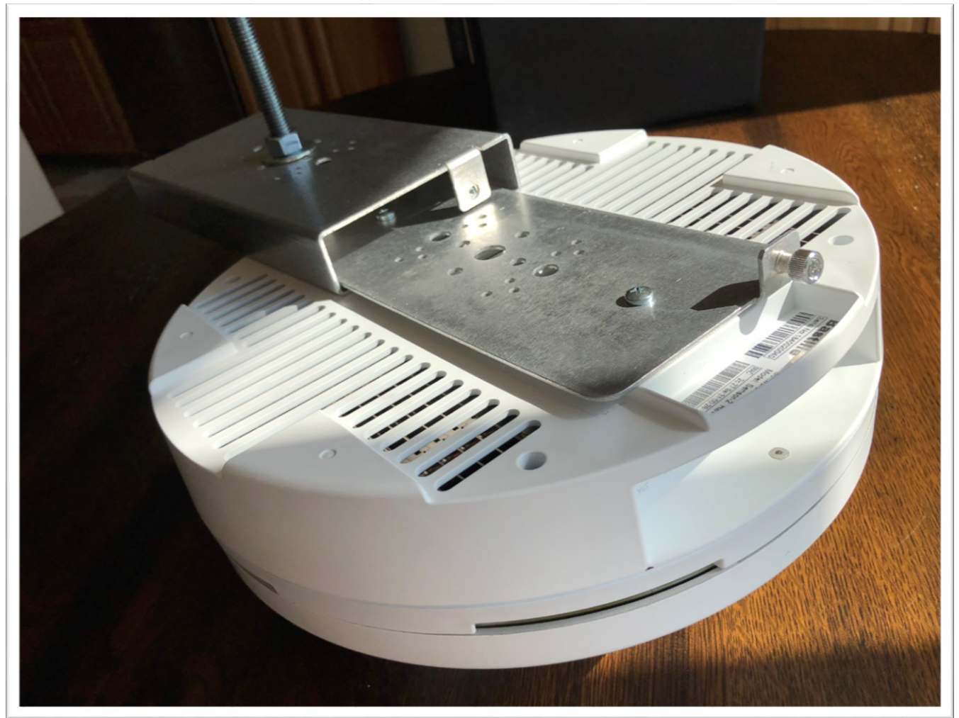
Figure 9. Insert Mounting Plate to Adapter Plate.
