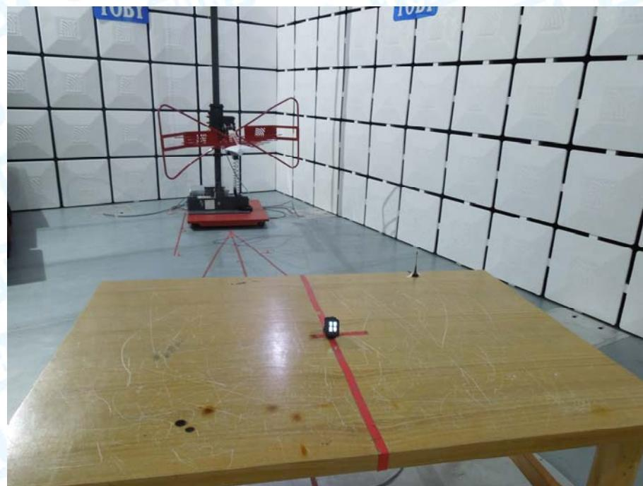
**Photo of Setup for Conducted Emission**
