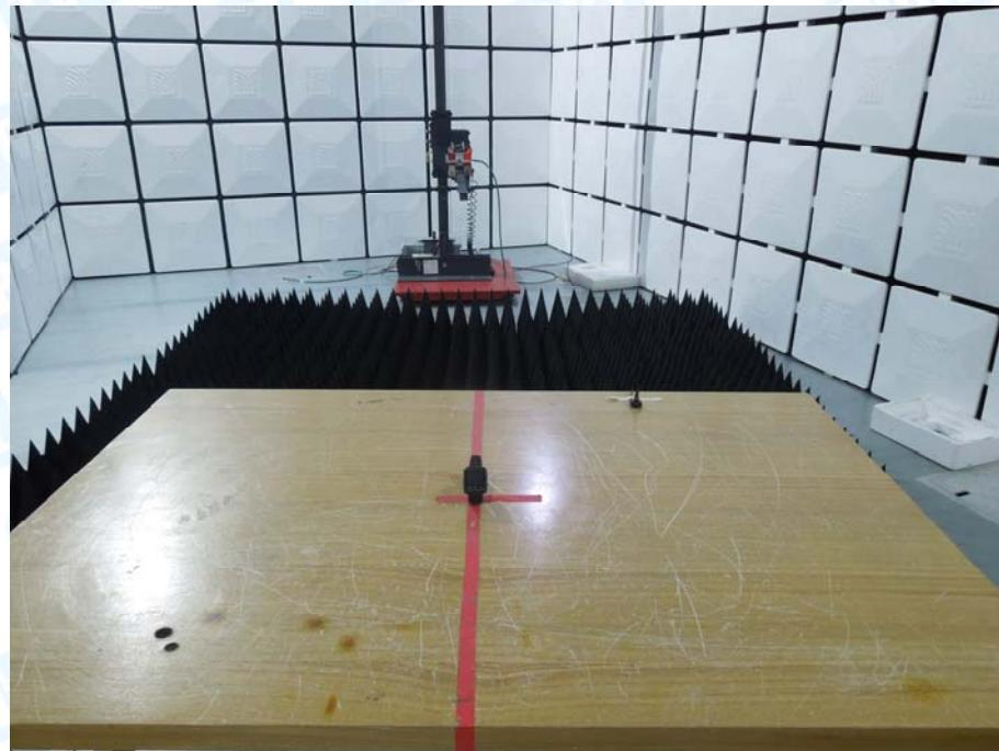
**Photo of Setup for Radiated Emission (Below 1 GHz)**
