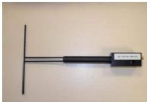
Figure 1 – Satimo COMOSAR Validation Dipole
