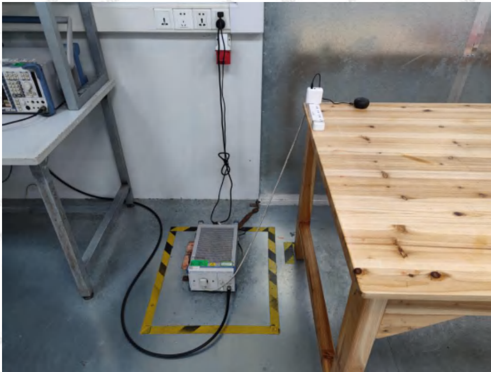
Photo of Power Line Conducted Emission Test
