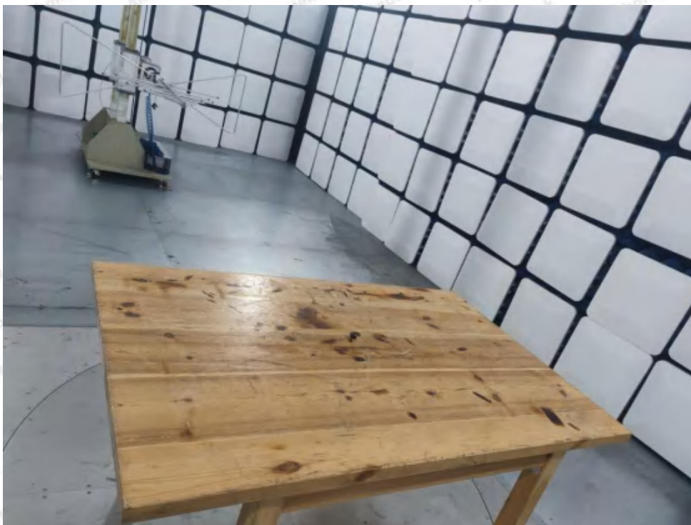
Photo of Radiation Emission Test
