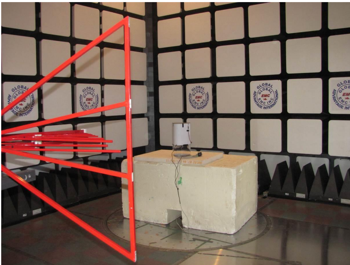
Figure 2: Radiated emission setup – photo 2
