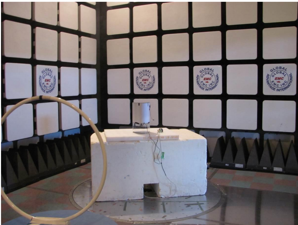
Figure 1: Radiated emissions setup – photo 1
