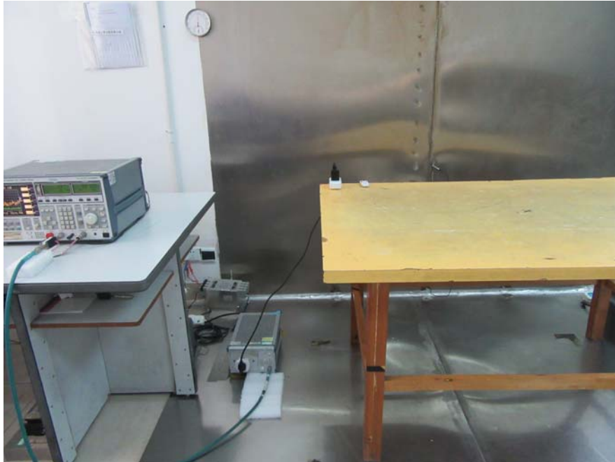
Conducted Emission Test Setup Front View
