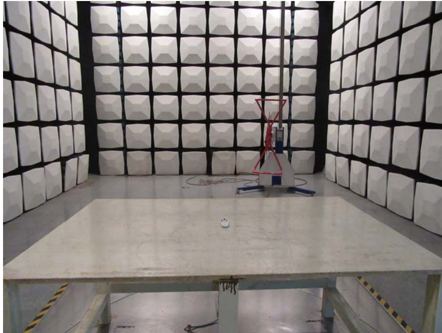
Radiated Disturbance Test Setup View (Below 1GHz)
