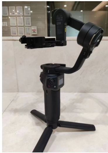
Locked state for installation(图 22)
