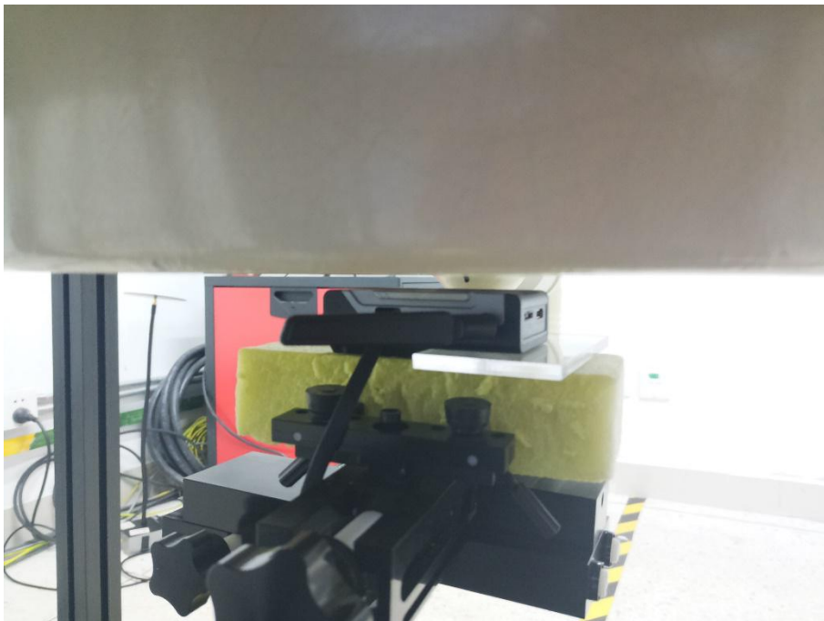
Front face of EUT with ANT A in open at 5mm (45 degrees)
