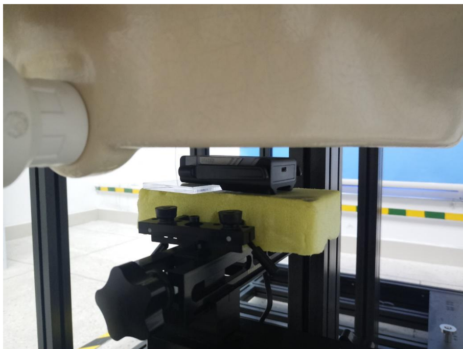
Front face of EUT with ANT B in close at 5mm (0 degrees)
