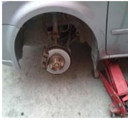
① Remove the tire ② Cut off the original valve of the car ③ Clean the valve hole ④ Installing sensors
