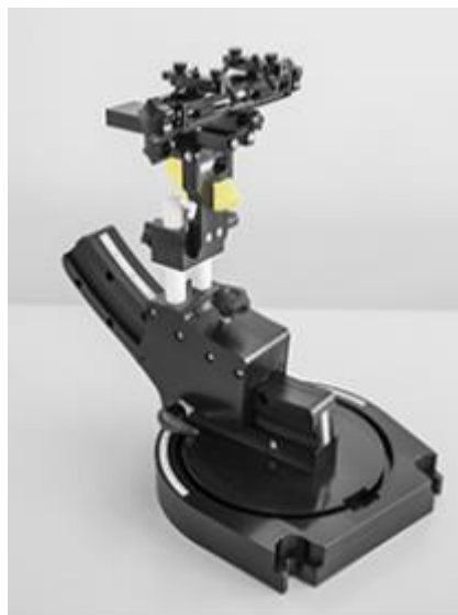
Device holder supplied by SPEAG
