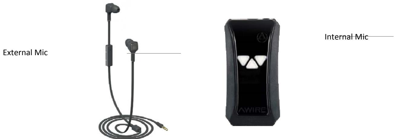
**AWIRE TIP:** Using the '*External Mic*' option will allow for clearer communication in situations where there is too much distance or interference between voice and the mic.
