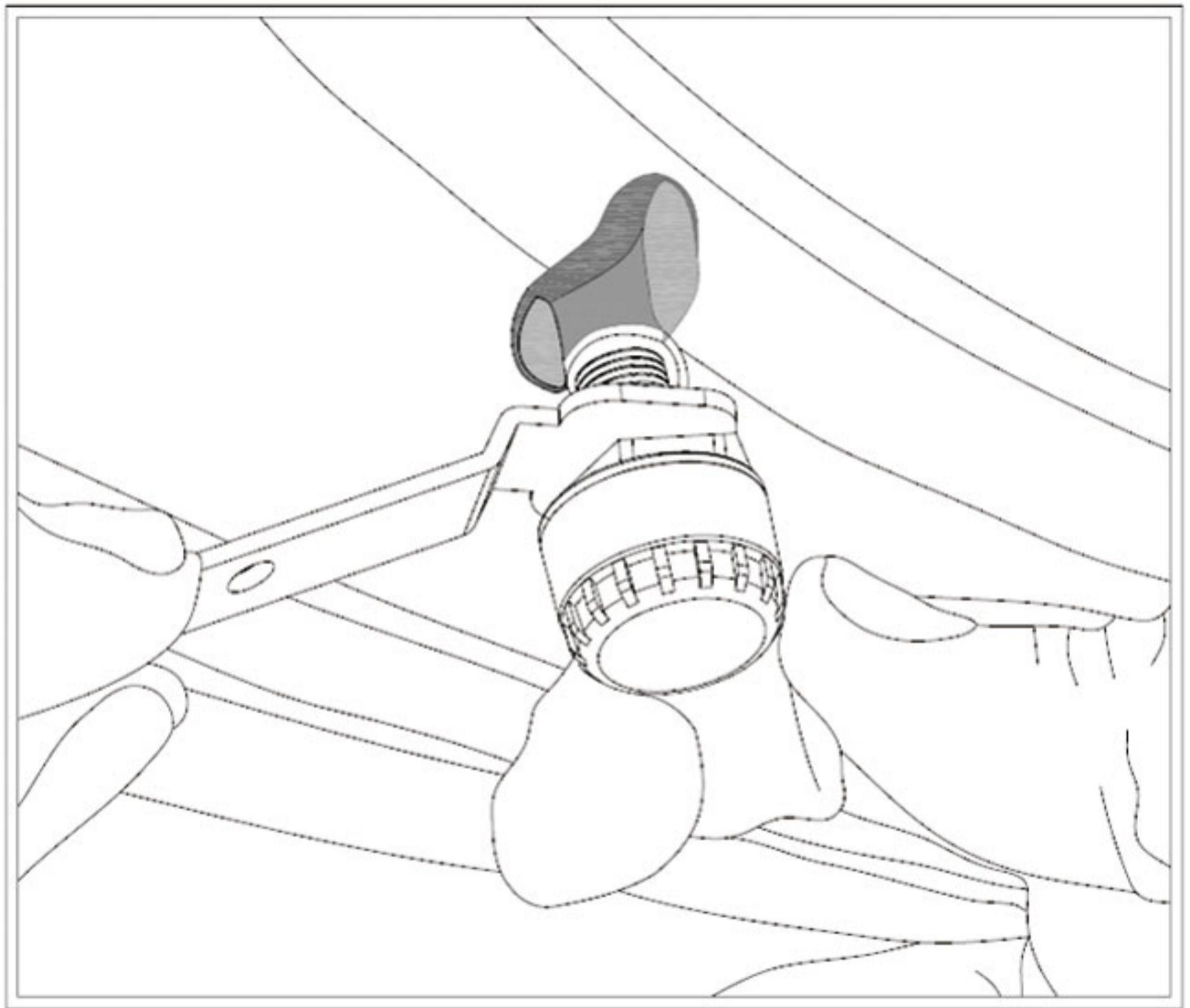
4 Use the wrench to tighten the washer by counter clock wide.
