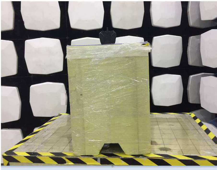
Above 1GHz (The EuT placed at the center of the turntable)
