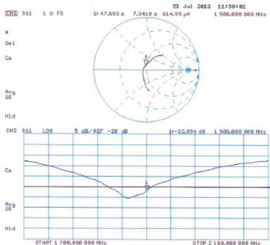
**D1900V2, Serial No.5d136 Extended Dipole Calibrations**
