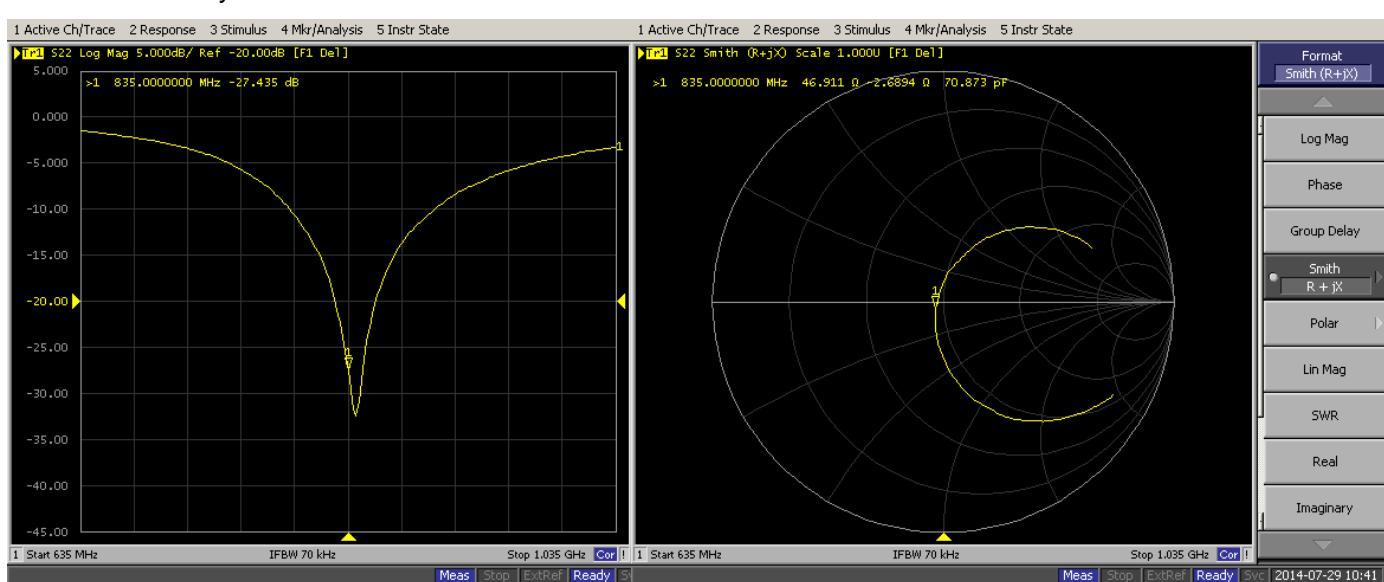
Per IEEE Std 1528-2013, the dipole should have a return loss better than -20dB at the test frequency to reduce uncertainty in the power measurement.
