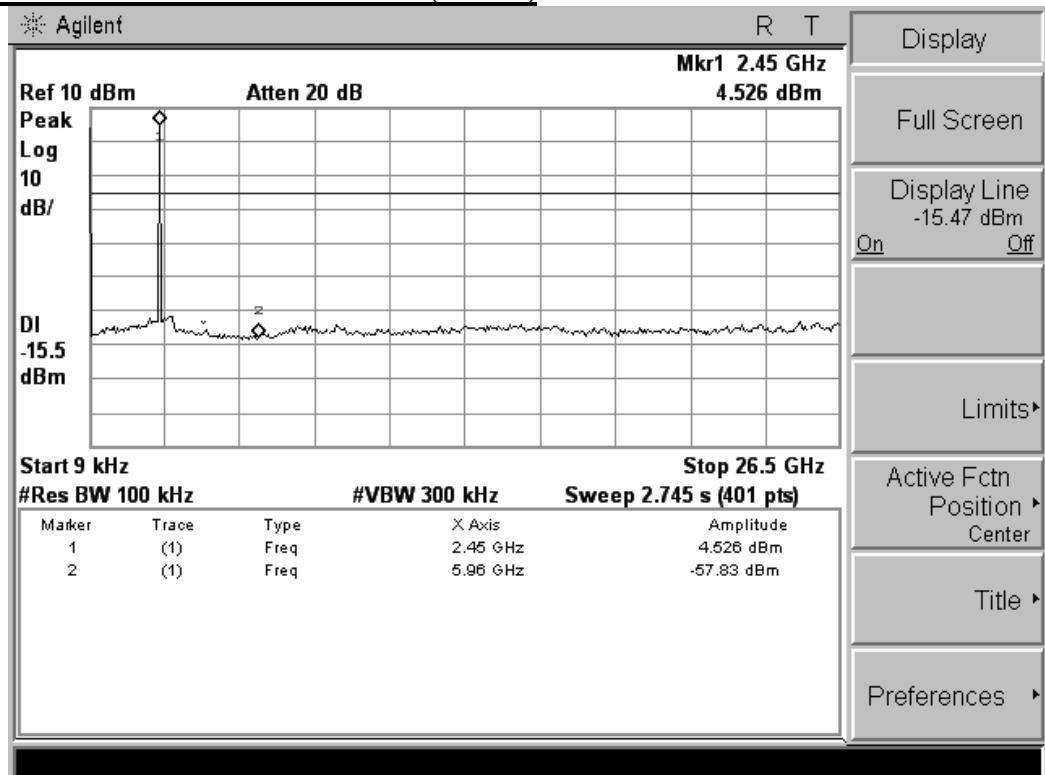
**9KHz-26.5GHz High Channel (GFSK)**
