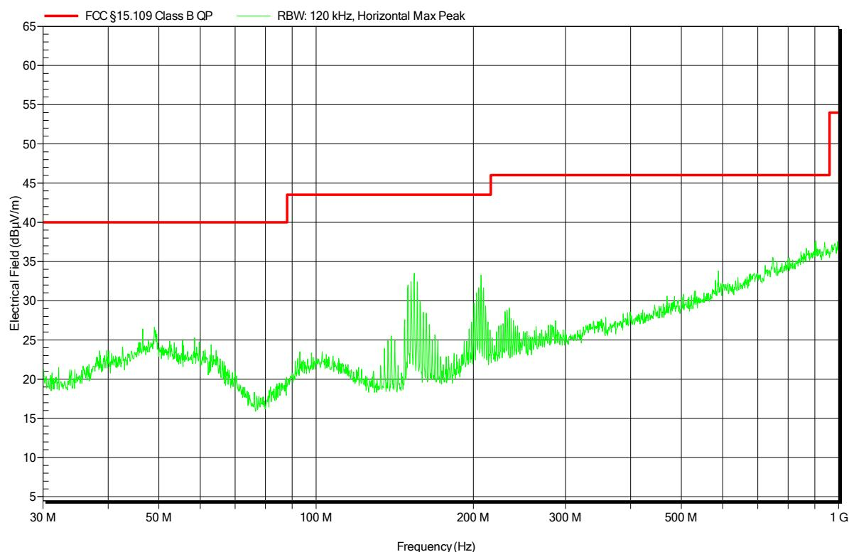
**Spurious emissions under normal conditions according to FCC 15B**
