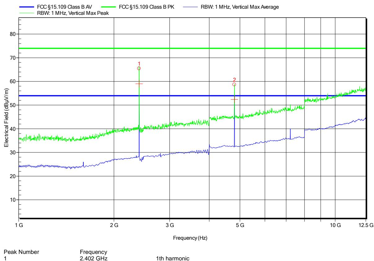
**Spurious emissions under normal conditions according to FCC 15B**
