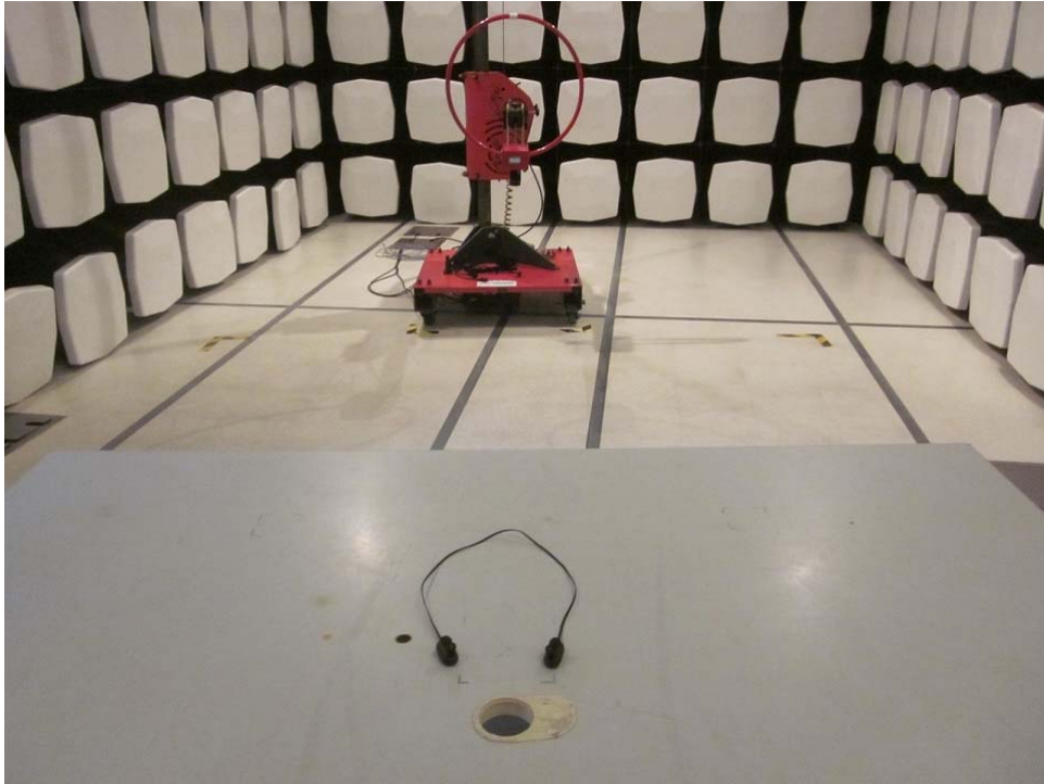
Measurement of Radiated Emission Test Set Up
