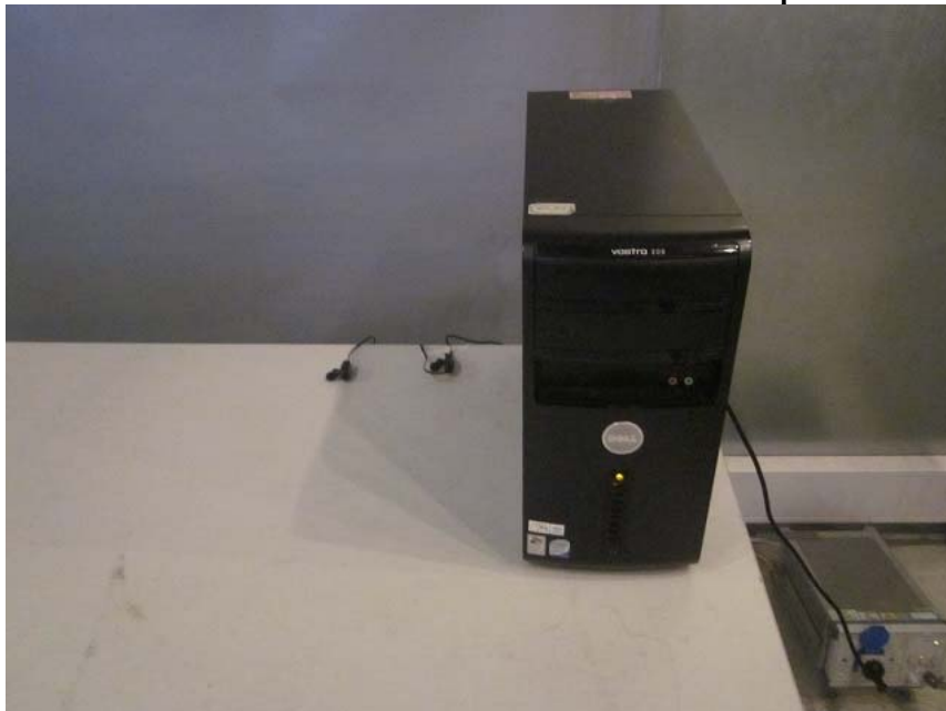
Measurement of Conducted Emission Test Set Up
