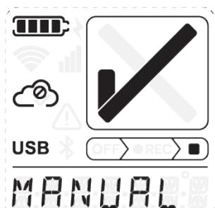
Device indicates that manual transfer of monitoring data to SmartView is required.
