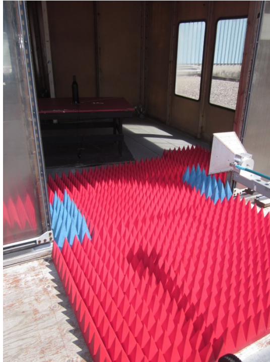
Wifi, Horizontal Antenna Polarization, 1 GHz to 12 GHz
