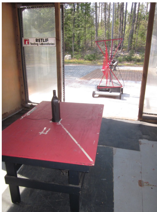
Wifi, Vertical Antenna Polarization, 30 MHz to 1 GHz
