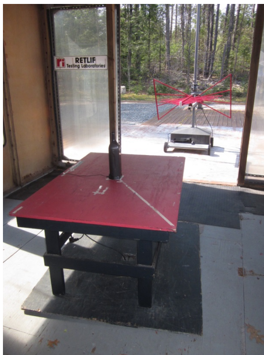
Wifi, Horizontal Antenna Polarization, 30 MHz to 1 GHz
