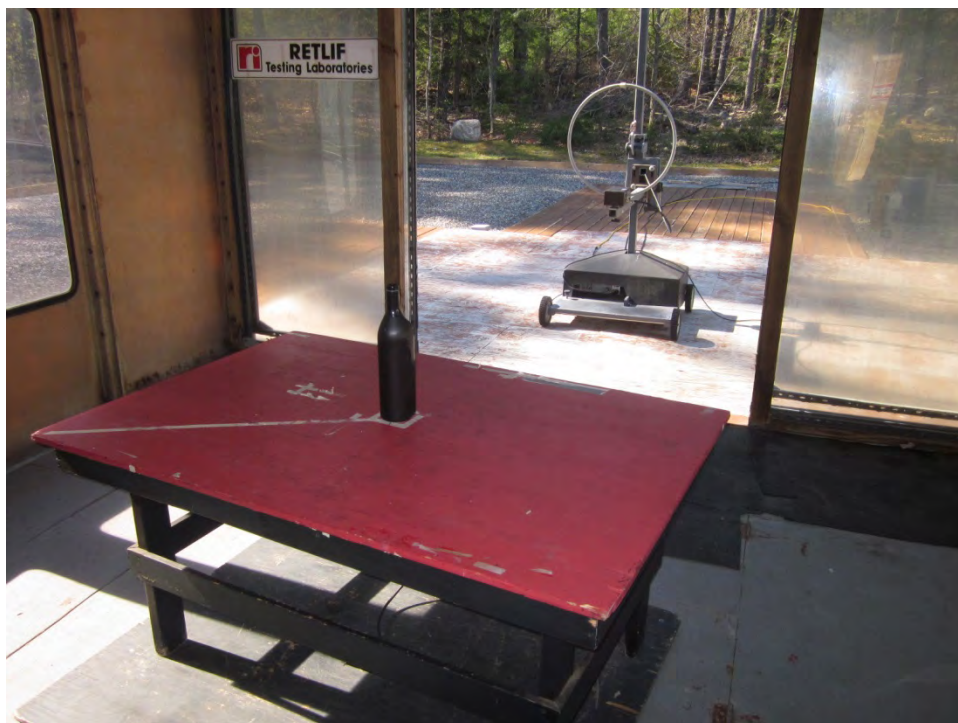
Test Setup, OATS, 9 kHz to 30 MHz
