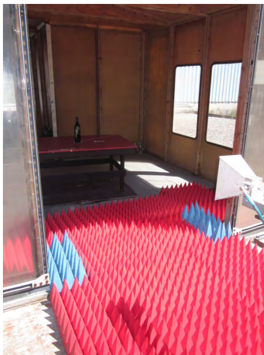
Test Setup, OATS, 1 to 5 GHz, Horizontal Antenna Polarization
