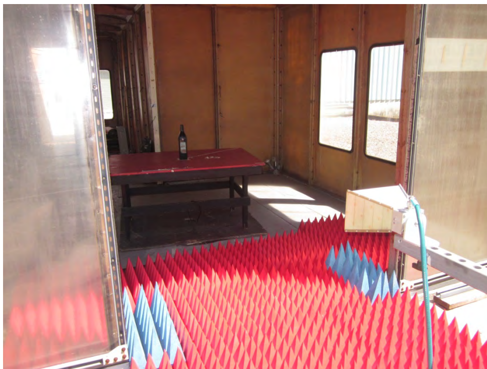
Test Setup, OATS, 1 to 5 GHz, Vertical Antenna Polarization
