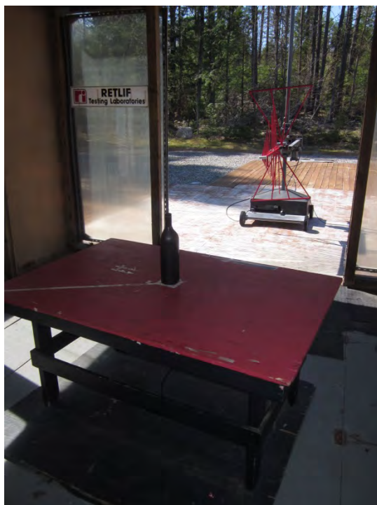
Test Setup, OATS, 30 MHz to 1 GHz, Vertical Antenna Polarization
