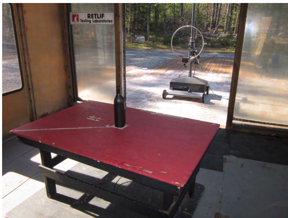
Test Setup, OATS, 9 kHz to 30 MHz
