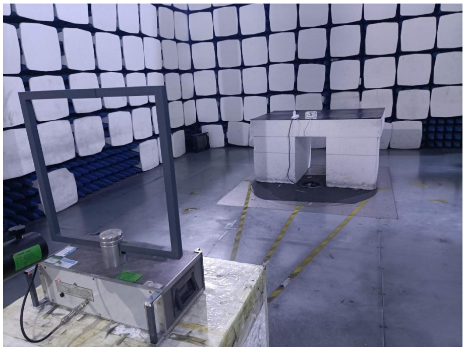
Radiation Emission Test Setup (Below 30MHz)
