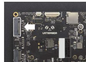
There are two M.2 sockets on the LattePanda Alpha& Delta, one M key and one E key. Both sockets have the 2280 size mounting screw.
