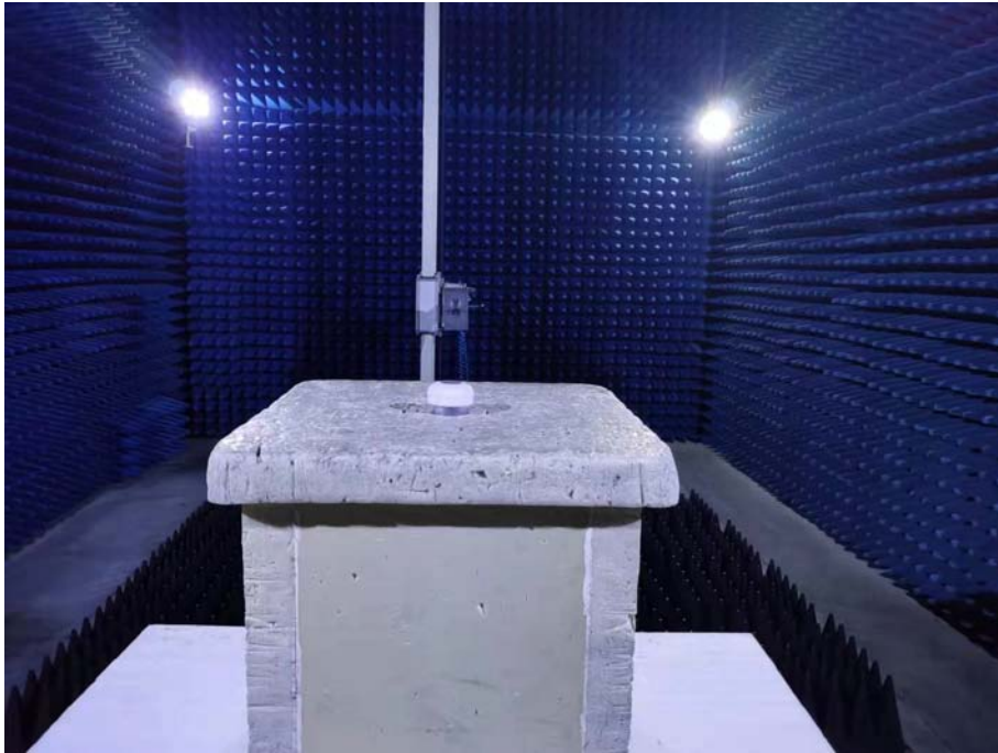
Photo of Radiated Emission Measurement Above 1GHz
