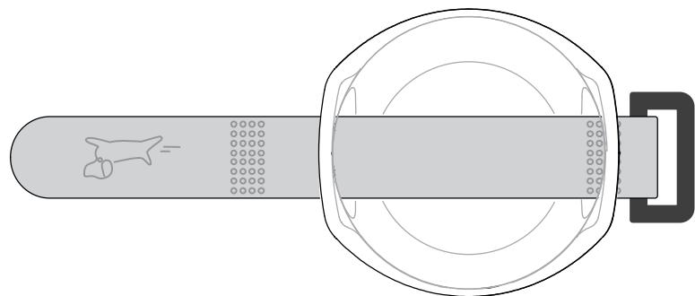
The fastener buckle is now fixed at one of the lugs. Next, take the loose edge of the fastener, fold it back towards the device and thread through the buckle.
