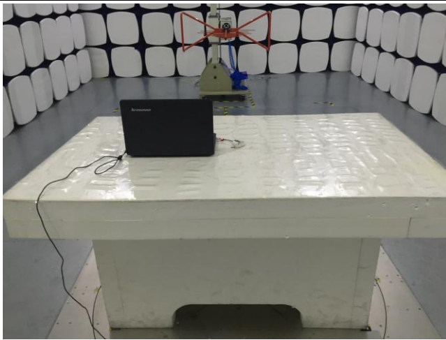
Radiated Spurious Emissions Test Setup Below 1GHz
