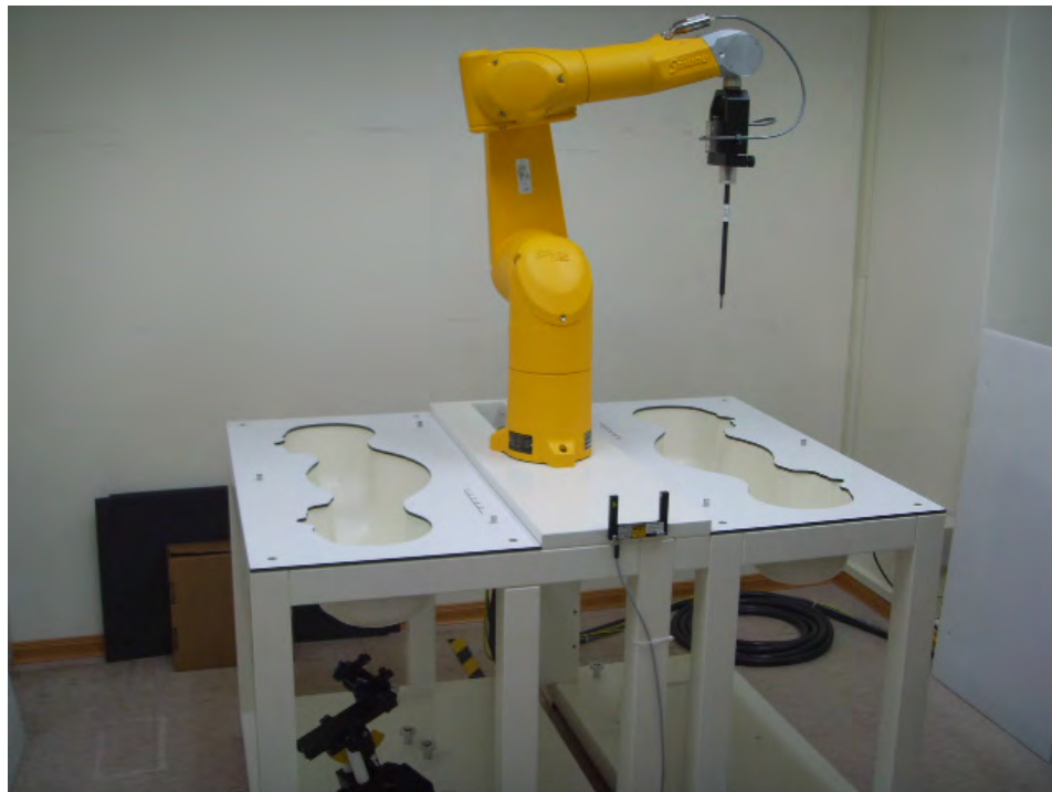
Fig.1 Photograph of the SAR measurement system
