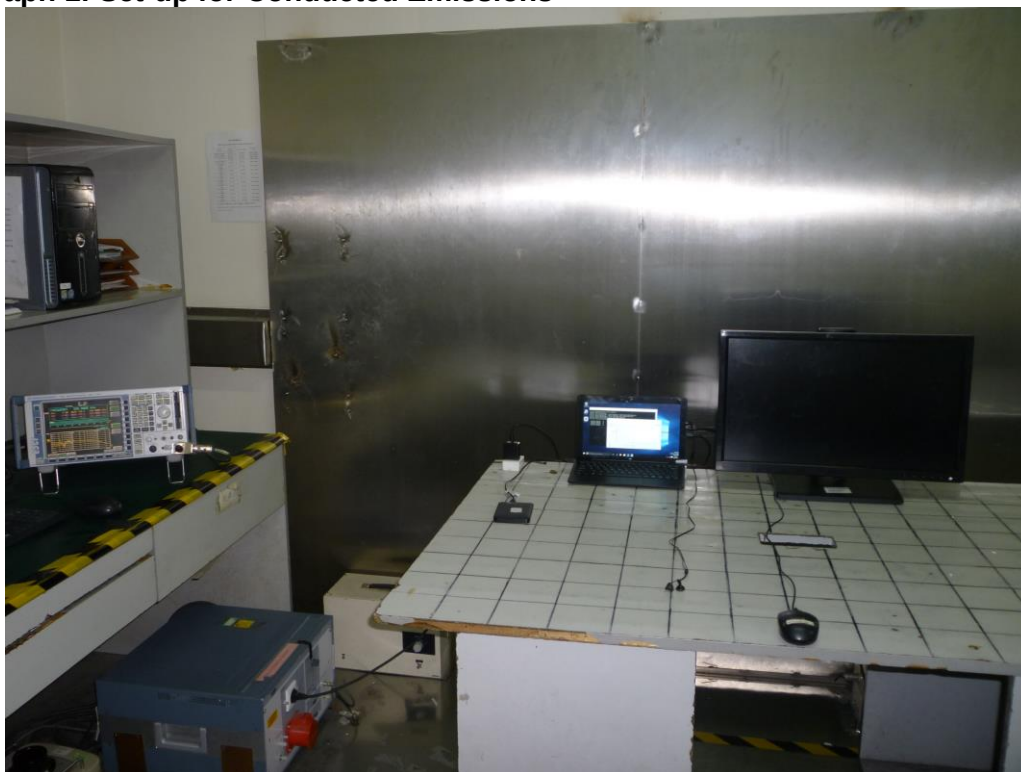
Photograph 2: Set-up for Spurious Emissions for 30 - 1000MHz
