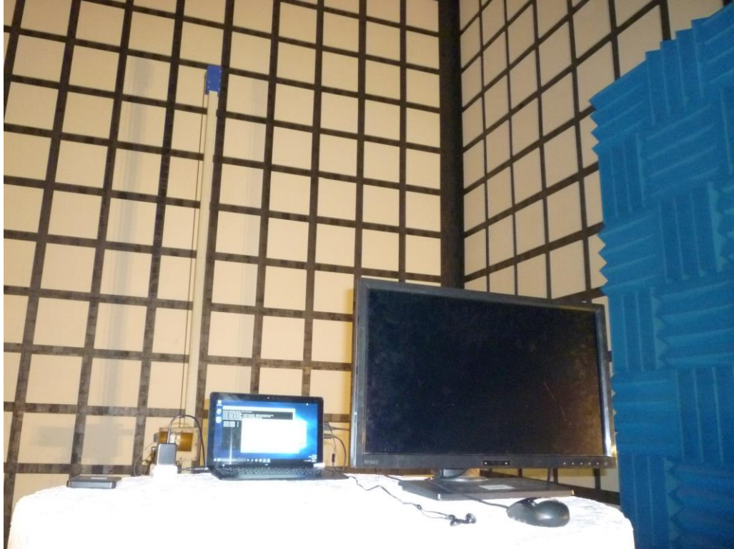
Photograph 4: Set-up for Dynamic Frequency Selection
