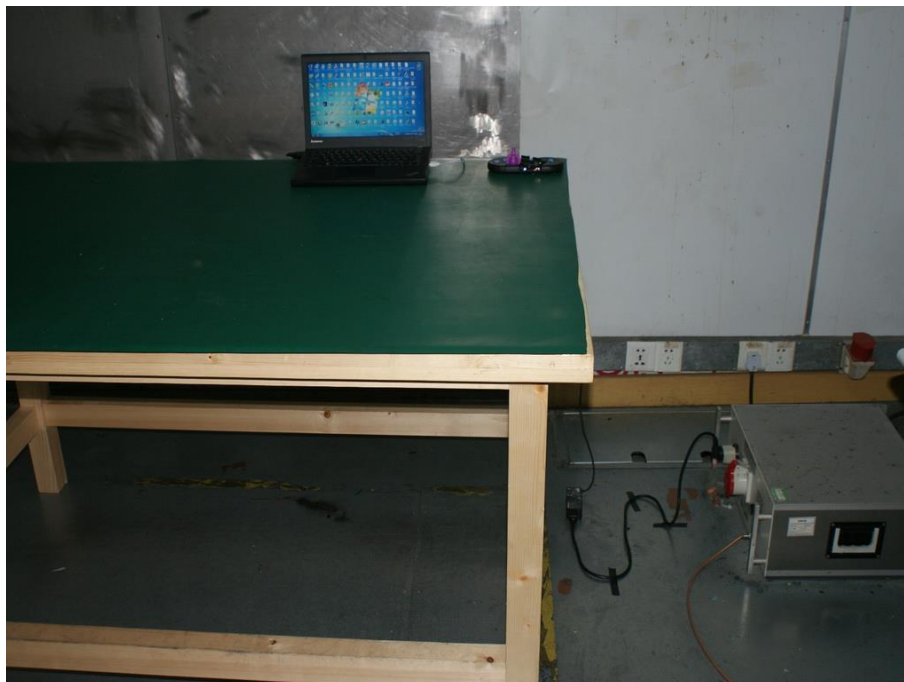
Photograph 6: Set-up for Conducted Emission on AC Mains
