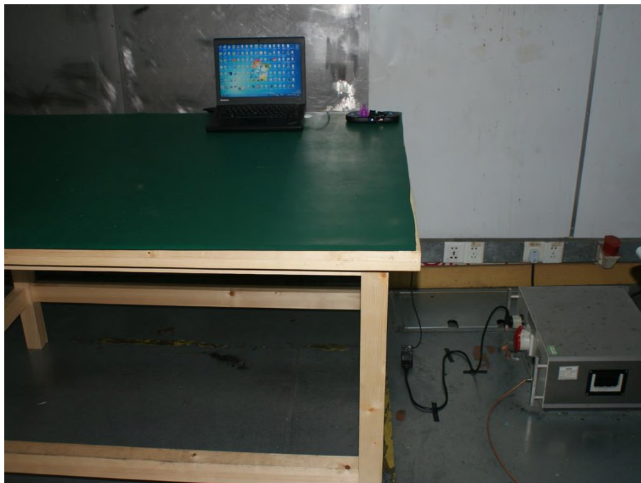
Photograph 6: Set-up for Conducted Emission on AC Mains
