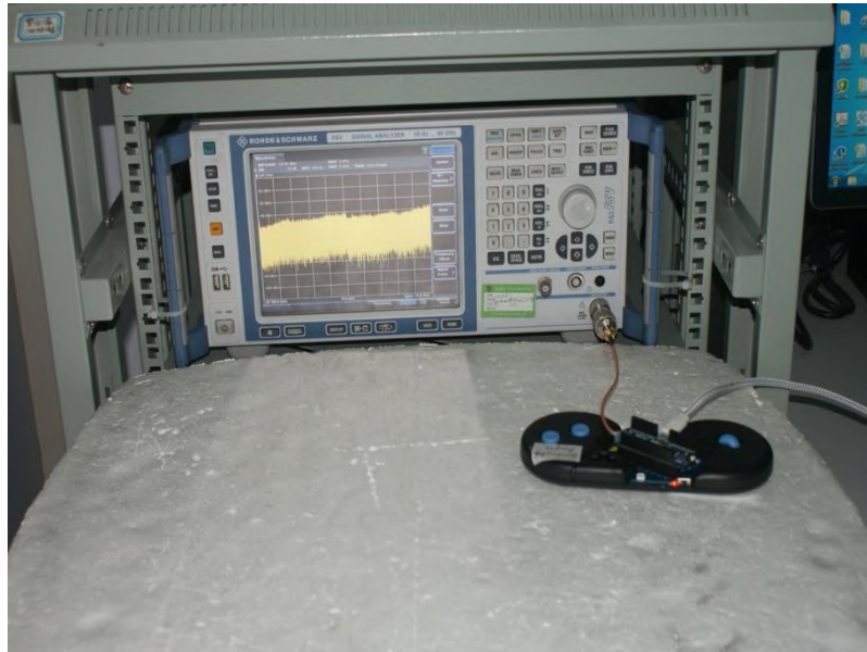
Photograph 1: Set-up for Radio Spectrum Test
