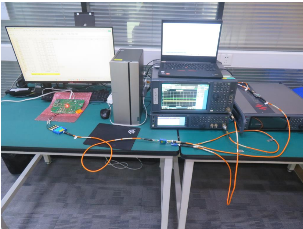
Description: Dynamic Frequency Selection Test Setup
