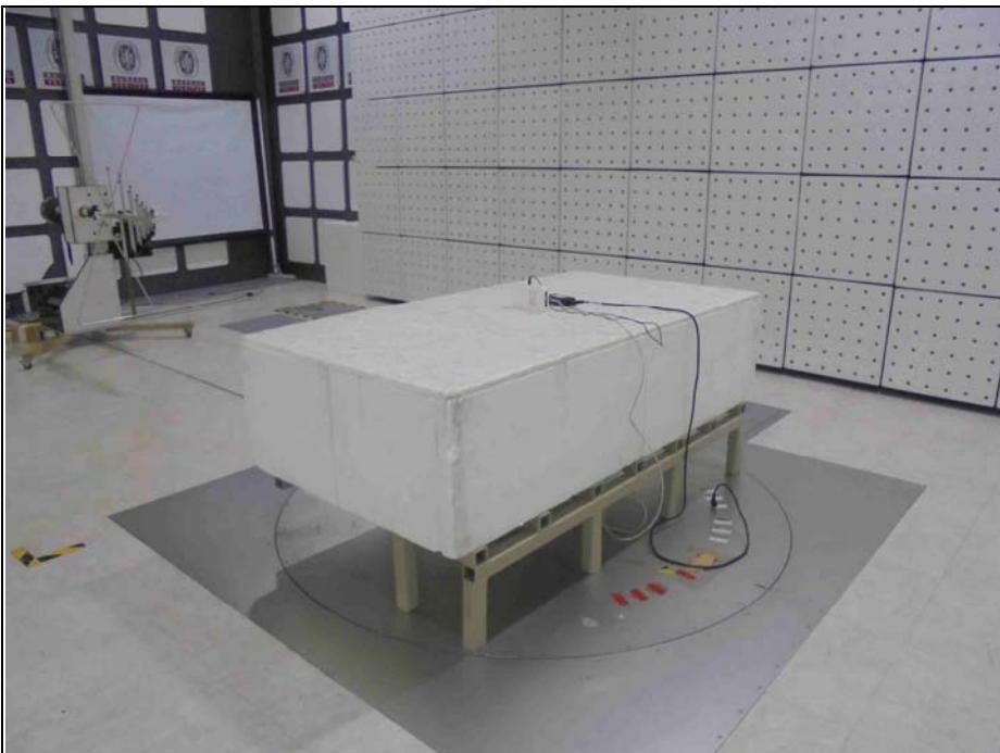
RADIATED EMISSION TEST (Mode A)
