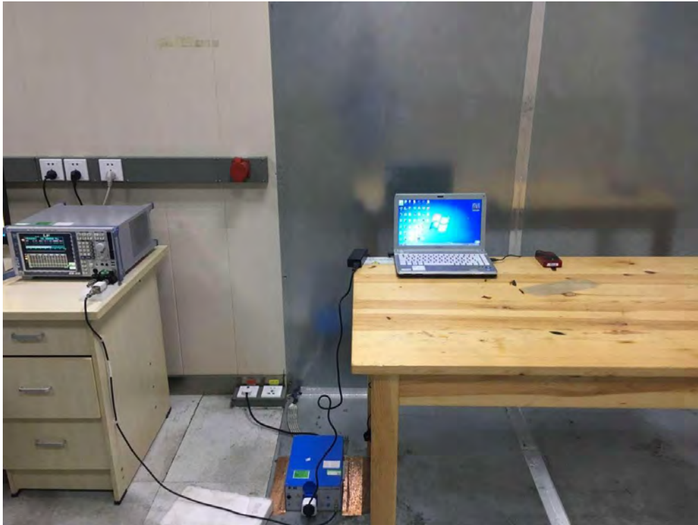
FCC RADIATED EMISSION TEST SETUP
