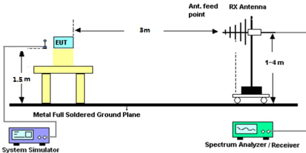
For radiated test from above 1GHz
