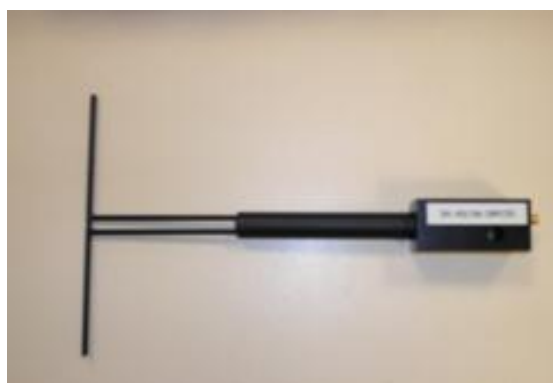
Figure 1 – Satimo COMOSAR Validation Dipole
