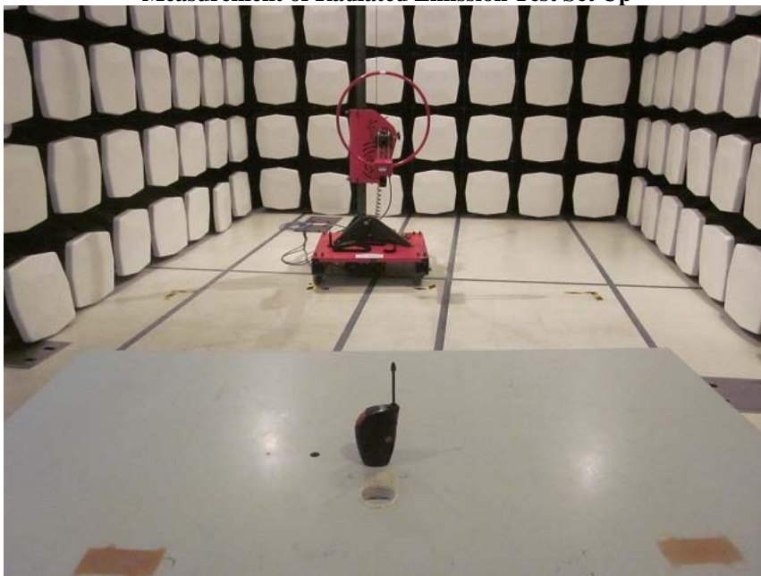
Measurement of Radiated Emission Test Set Up
