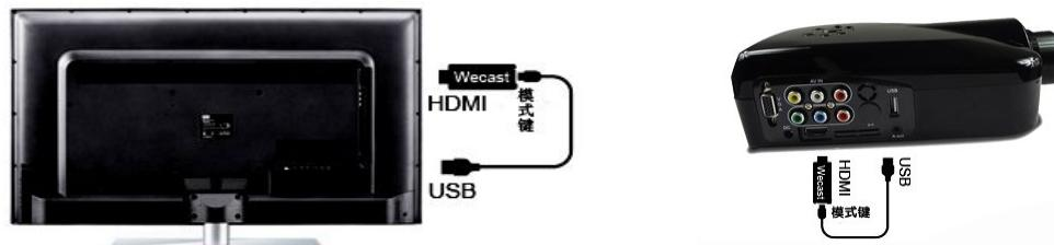
Note: pls check whether the USB Port of TV or projector is workable or not. If not, pls use USB cable to connect the USB power adapter to charge the dongle.
