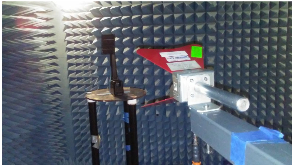
Photograph 1. Radiated Spurious Emissions, Test Setup Above 1GHz
