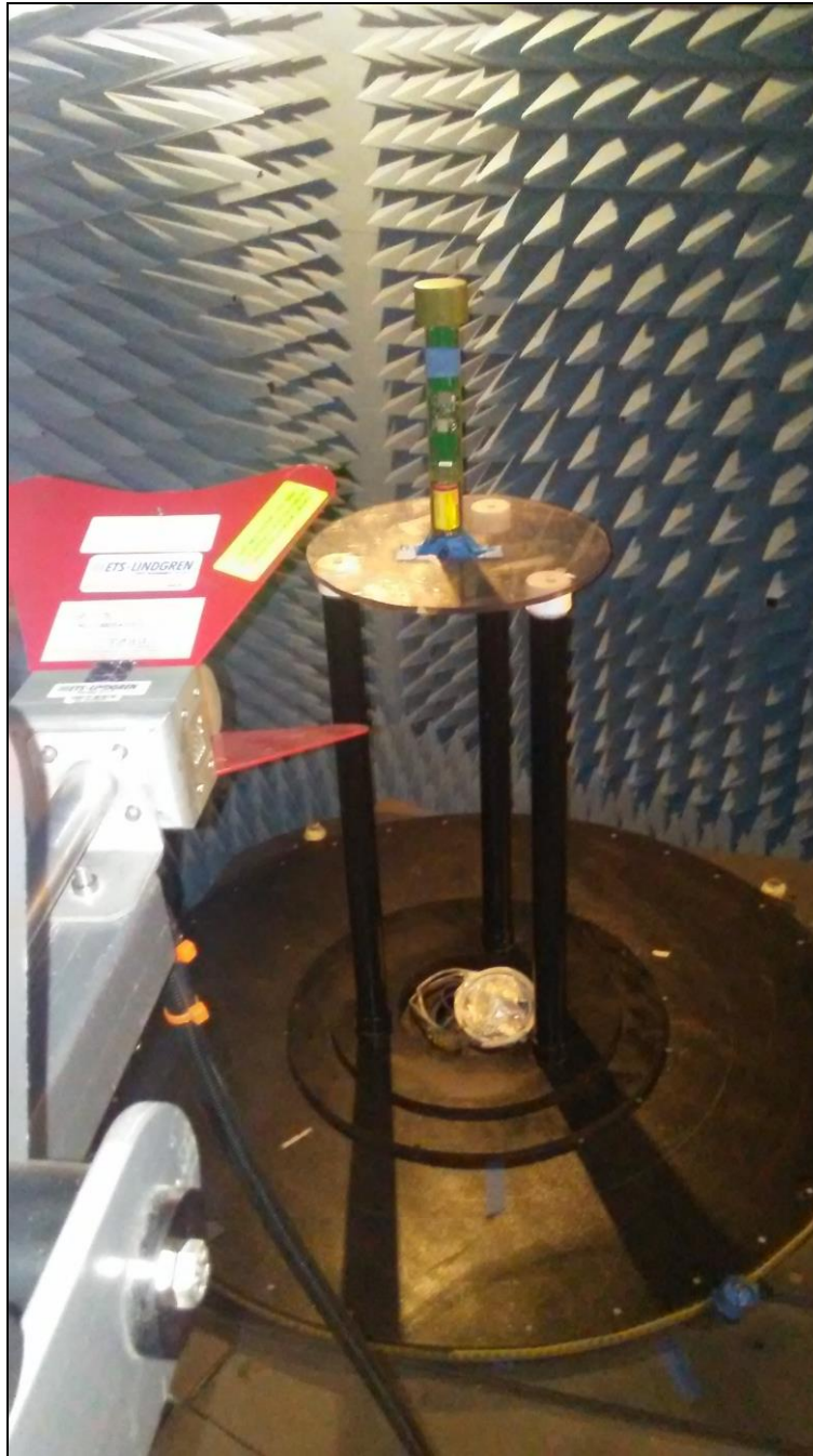
Photograph 2. Radiated Spurious Emissions Setup, Above 1GHz
