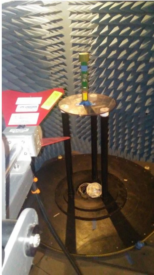
Photograph 4. Radiated Spurious Emissions, Above 1GHz, Test Setup
