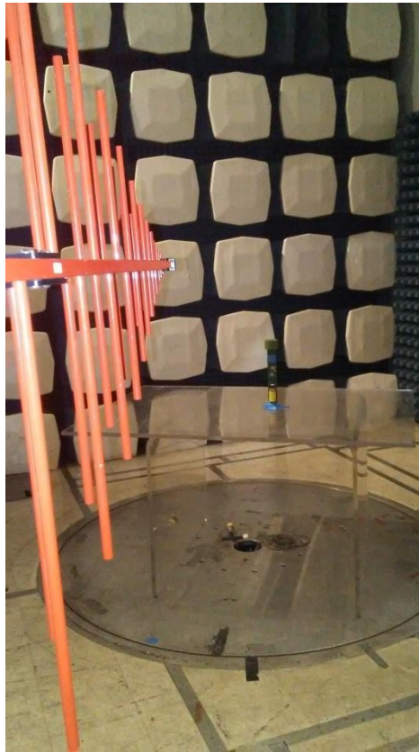
Photograph 3. Radiated Spurious Emissions, Below 1GHz, Test Setup
