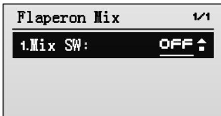
2. Modify the value of **Mix SW** to **ON** by pressing **R/+** key, to activate Flaperon mixing function.
