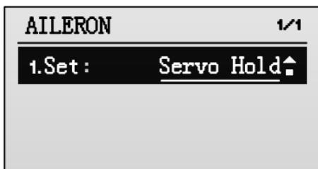
3. Change the value to **Fail Safe** by pressing **R/+** key, to activate fail safe function.
