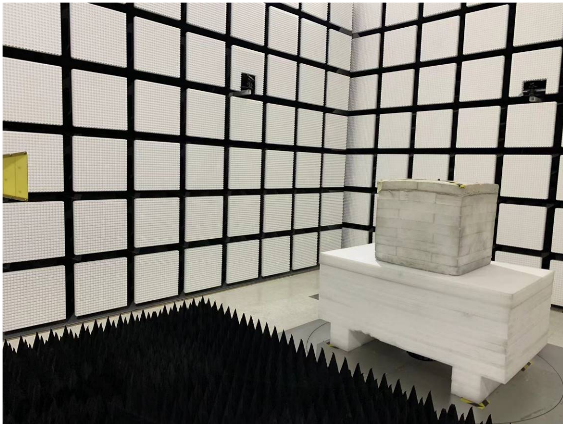
Radiated Emission Above 1GHz View
